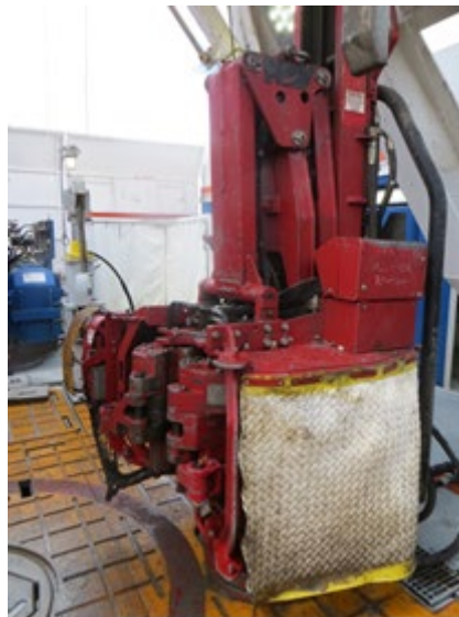
Figure 10: Iron Roughneck, an Example of Rig Mechanization
