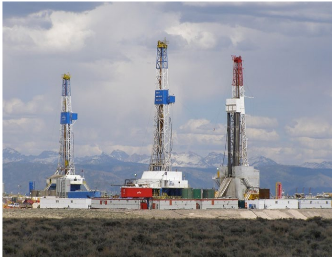
Figure 2: Petroleum Rig Operations (Pad Drilling in the Rockies)
